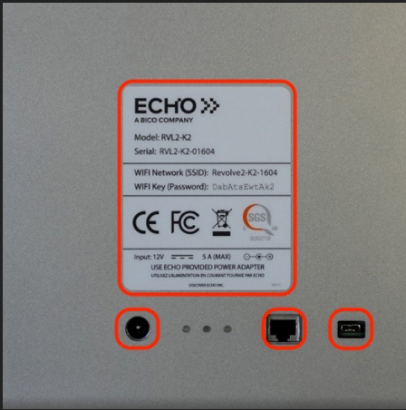
Rear panel of the Revolve Microscope. The sticker with the Serial Number and Wi-Fi Network (SSID and Password), along with the power, ethernet, and USB-C ports are highlighted.
