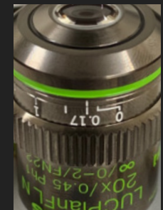
20x Phase Objective with a correction collar set to 0.17.
